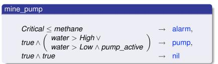
From this it is easy to see that the pump is only ever active while the methane level is not critical and the water level is at least above low.
